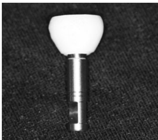
Figure 3 Sample of a full-coverage ceramic test restoration fabricated using the CEREC 3D system. The occlusal surface has been modified to fit the securing jig of the instron machine.
